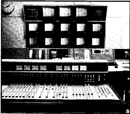
View from operating seat of sound engineer at TV-master control room (Studer 369 special)
