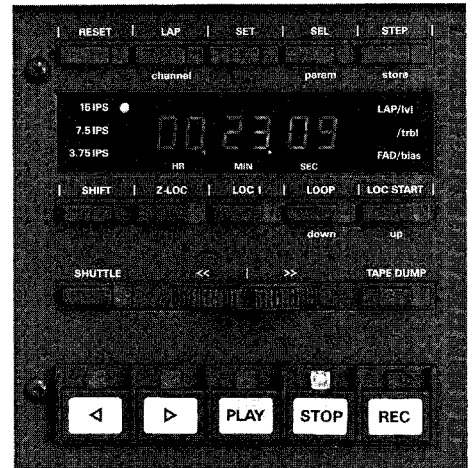
Multifunctional: Tape counter and transport functions.
