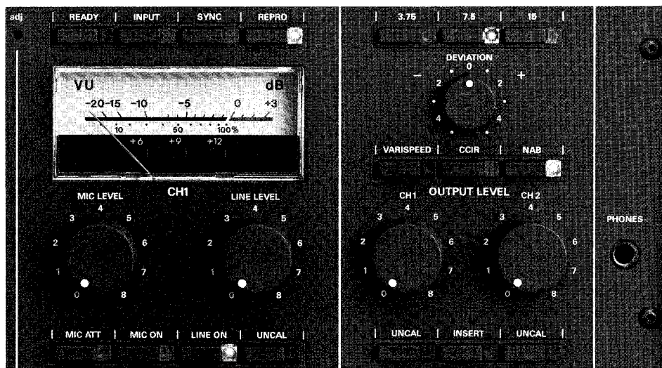
Comprehensive operating facilities for every application. VU-meter with integrated peak indicators.
